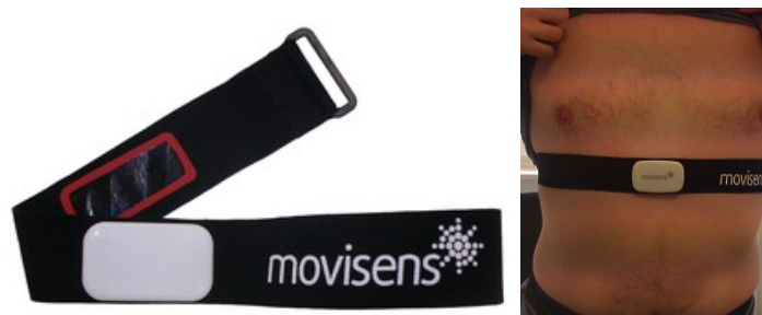
Fig. 1. The Movisens sensor and the sensor belt: On the inside of the sensor belt one of the two dry electrodes is visible. The sensor's battery supports 24 hours of recording ECG and acceleration data.
